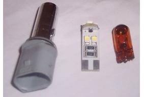
**Step 8:** Remove the stock orange bulb and insert the LED. Notice you won't know what polarity is which, so you must test the vehicle with the bulb dangling from the fender well to see if you got the correct polarity. Otherwise, if wrong polarity, the bulb won't turn on. LED are polarities sensitive.
